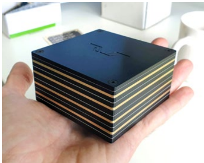
Figure 12 Rosella 0.5 U enclosure mock-up showing interleaved PCBs and aluminium enclosure walls (credit: ANU)
