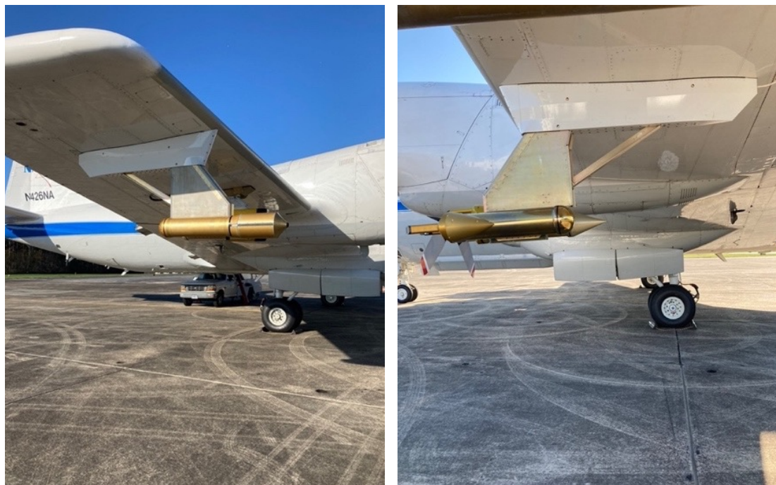
Figure 43. New P-3 wing pylons carrying canister probes for the IMPACTS mission. Photo credit: NASA
