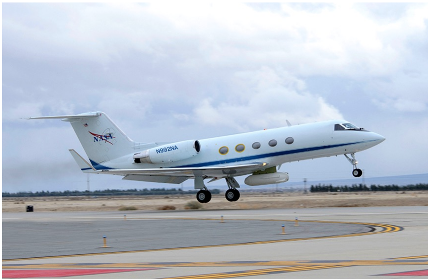
Figure 53. The JSC G-III taking flight to collect data. The P-band radar pod is mounted underneath. Photo credit: Tony Landis
